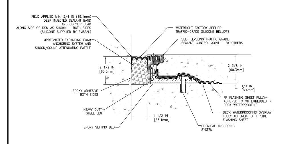
MOVEMENT: ±50% + 3/4 IN (19mm) - 3/4 IN (19mm)
