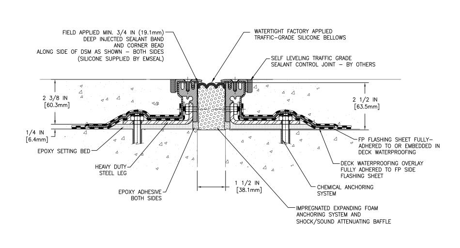
MOVEMENT: ±50% + 3/4 IN (19mm) - 3/4 IN (19mm)
