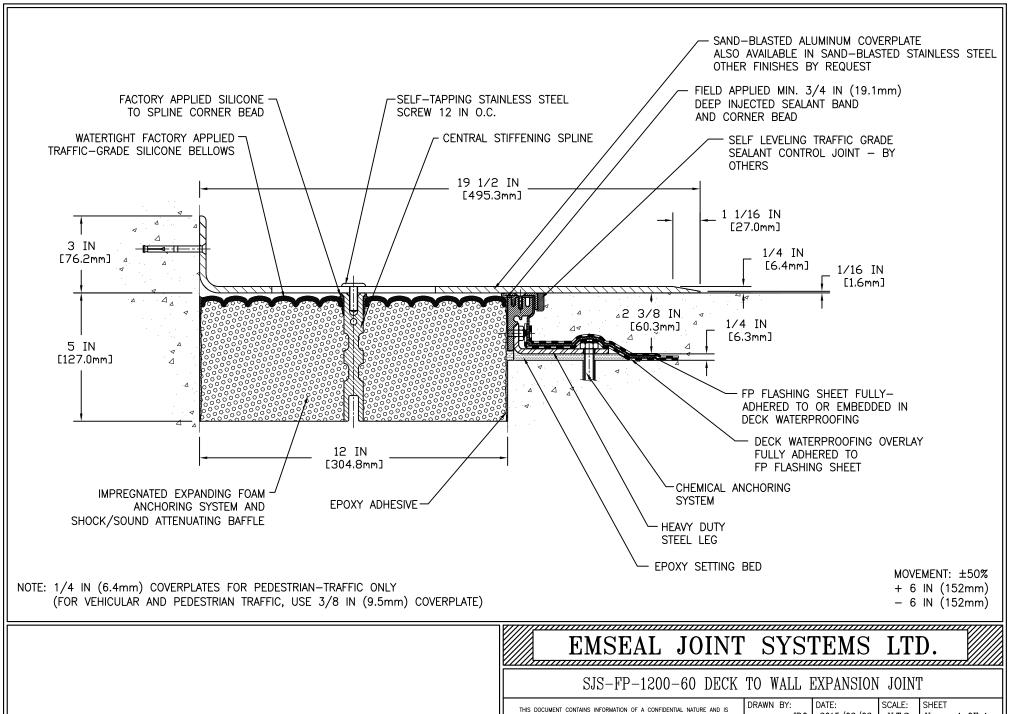
THIS DOCUMENT CONTAINS INFORMATION OF A CONFIDENTIAL NATURE AND IS PROPRIETARY TO EMERAL JOINT SYSTEMS LTD. AND UNAUTHORIZED USE WILL BE PROSECULED. THIS DRAWING IS PROTECTED BY COPYRIGHT, THE RIGHT TO REPRODUCE IN ANY FORM BEING THE EXCLUSIVE RIGHT OF EMERAL JOINT SYSTEMS LTD. ANY UNAUTHORIZED REPRODUCTION WHETHER IN TWO OR THREE DIMENSIONS WILL BE PROSECUTED. © 2014 EMSEAL JOINT SYSTEMS LTD.
