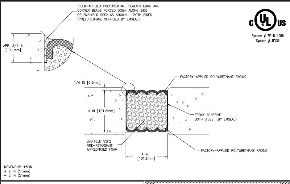
EMSEAL'S EMSHIELD SSF2 HAS BEEN TESTED IN ACCORDANCE WITH UL 2079 IN THE CONFIGURATION DEPICTED IN SYSTEM # FF-D-1089. USE OF THIS MATERIAL IN WALL ASSEMBLY CONFIGURATIONS OTHER THAT DEPICTED IN UL SYSTEM # FF-D-1089 WILL NOT ENCUMBER OR LOWER THE RESISTANCE OF THE WALL BUT IS DONE SO AT THE DESIGNERS' DISCRETION AND RESPONSIBILITY FOR DESIGN OF A FIRE RATED WALL ASSEMBLY THAT MEETS APPLICABLE STANDARDS FOR THE PROJECT AND WHICH ADDITIONALLY IS CAPABLE OF RESISTING THE APPROXIMATELY 2.5 PSI
