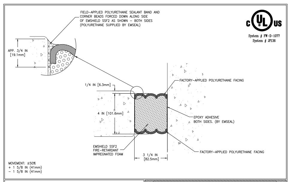
EMSEAL'S EMSHIELD SSF2 HAS BEEN TESTED IN ACCORDANCE WITH UL 2079 IN THE CONFIGURATION DEPICTED IN SYSTEM # FW-D-1077. USE OF THIS MATERIAL IN WALL ASSEMBLY CONFIGURATIONS OTHER THAT DEPICTED IN UL SYSTEM # FW-D-1077 WILL NOT ENCUMBER OR LOWER THE RESISTANCE OF THE WALL BUT IS DONE SO AT THE DESIGNERS' DISCRETION AND RESPONSIBILITY FOR DESIGN OF A FIRE RATED WALL ASSEMBLY THAT MEETS APPLICABLE STANDARDS FOR THE PROJECT AND WHICH ADDITIONALLY IS CAPABLE OF RESISTING THE APPROXIMATELY 2.5 PSI
