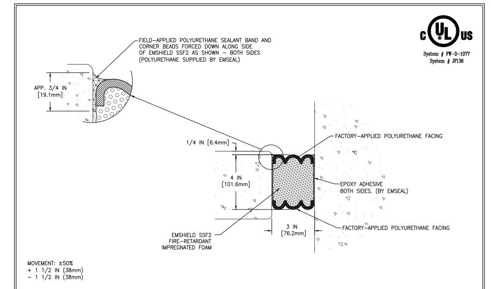
EMSEAL'S EMSHIELD SSF2 HAS BEEN TESTED IN ACCORDANCE WITH UL 2079 IN THE CONFIGURATION DEPICTED IN SYSTEM # FF-D-1089. USE OF THIS MATERIAL IN WALL ASSEMBLY CONFIGURATIONS OTHER THAT DEPICTED IN UL SYSTEM # FF-D-1089 WILL NOT ENCUMBER OR LOWER THE RESISTANCE OF THE WALL BUT IS DONE SO AT THE DESIGNERS' DISCRETION AND RESPONSIBILITY FOR DESIGN OF A FIRE RATED WALL ASSEMBLY THAT MEETS APPLICABLE STANDARDS FOR THE PROJECT AND WHICH ADDITIONALLY IS CAPABLE OF RESISTING THE APPROXIMATELY 2.5 PSI
