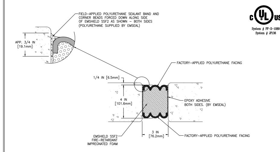
MOVEMENT: ±50% + 1 1/2 IN (38mm) - 1 1/2 IN (38mm)
