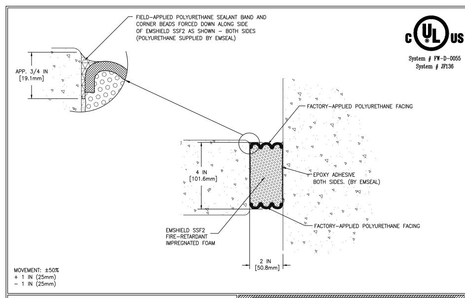
EMSEAL'S EMSHIELD SSF2 HAS BEEN TESTED IN ACCORDANCE WITH UL 2079 IN THE CONFIGURATION DEPICTED IN SYSTEM # FW-D-0055. USE OF THIS MATERIAL IN WALL ASSEMBLY CONFIGURATIONS OTHER THAT DEPICTED IN UL SYSTEM # FW-D-0055 WILL NOT ENCUMBER OR LOWER THE RESISTANCE OF THE WALL BUT IS DONE SO AT THE DESIGNERS' DISCRETION AND RESPONSIBILITY FOR DESIGN OF A FIRE RATED WALL ASSEMBLY THAT MEETS APPLICABLE STANDARDS FOR THE PROJECT AND WHICH ADDITIONALLY IS CAPABLE OF RESISTING THE APPROXIMATELY 2.5 PSI
