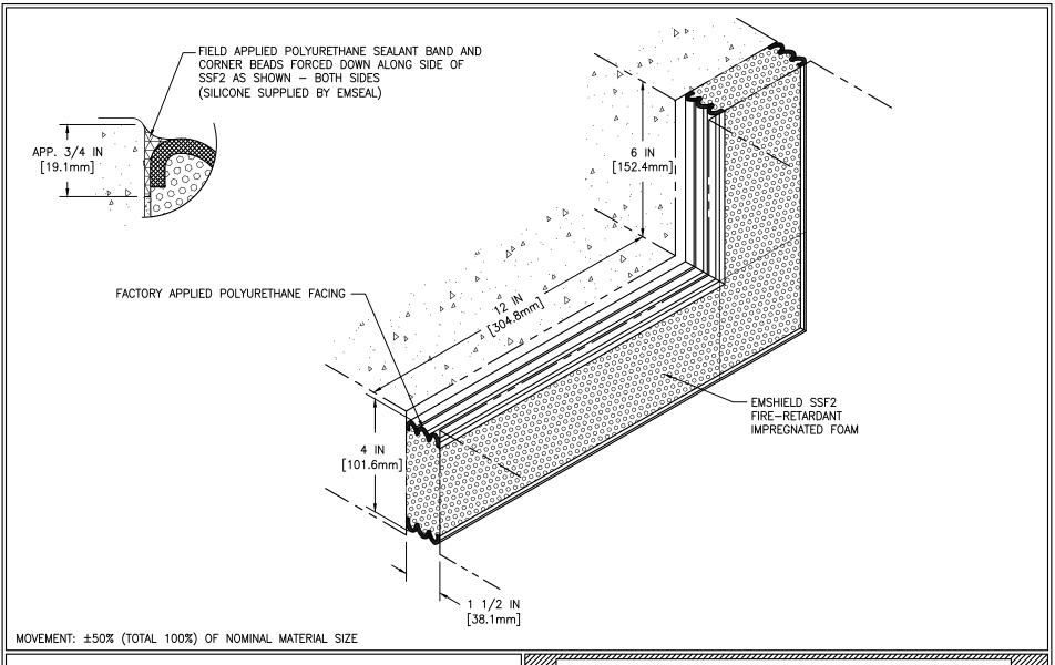
EMSEAL'S EMSHIELD SSF2 HAS BEEN TESTED IN ACCORDANCE WITH UL 2079 IN THE CONFIGURATION DEPICTED IN SYSTEM # FF-D-0077. USE OF THIS MATERIAL IN WALL ASSEMBLY CONFIGURATIONS OTHER THAT DEPICTED IN UL SYSTEM # FF-D-0077 WILL NOT ENCUMBER OR LOWER THE RESISTANCE OF THE WALL BUT IS DONE SO AT THE DESIGNERS' DISCRETION AND RESPONSIBILITY OR DESIGN OF A FIRE RATED WALL ASSEMBLY THAT MEETS APPLICABLE STANDARDS FOR THE PROJECT AND WHICH ADDITIONALLY IS CAPABLE OF RESISTING THE APPROXIMATELY 2.5 PSI
