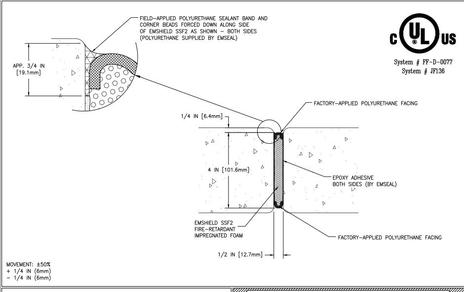
EMSEAL'S EMSHIELD SSF2 HAS BEEN TESTED IN ACCORDANCE WITH UL 2079 IN THE CONFIGURATION DEPICTED IN SYSTEM # FF-D-0077. USE OF THIS MATERIAL IN WALL ASSEMBLY CONFIGURATIONS OTHER THAT DEPICTED IN UL SYSTEM # FF-D-0077 WILL NOT ENCUMBER OR LOWER THE RESISTANCE OF THE WALL BUT IS DONE SO AT THE DESIGNERS' DISCRETION AND RESPONSIBILITY FOR DESIGN OF A FIRE RATED WALL ASSEMBLY THAT MEETS APPLICABLE STANDARDS FOR THE PROJECT AND WHICH ADDITIONALLY IS CAPABLE OF RESISTING THE APPROXIMATELY 2.5 PSI
