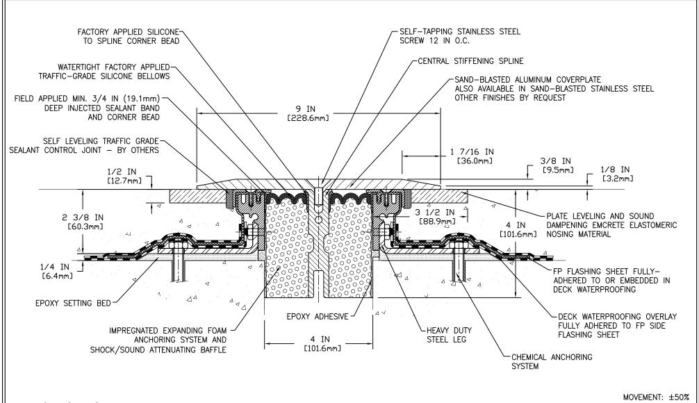
NOTE: 3/8 IN (9.5mm) COVERPLATES FOR VEHICLE AND PEDESTRIAN—TRAFFIC USE (FOR PEDESTRIAN—TRAFFIC ONLY, USE 1/4 IN (6.4mm) COVERPLATE)
