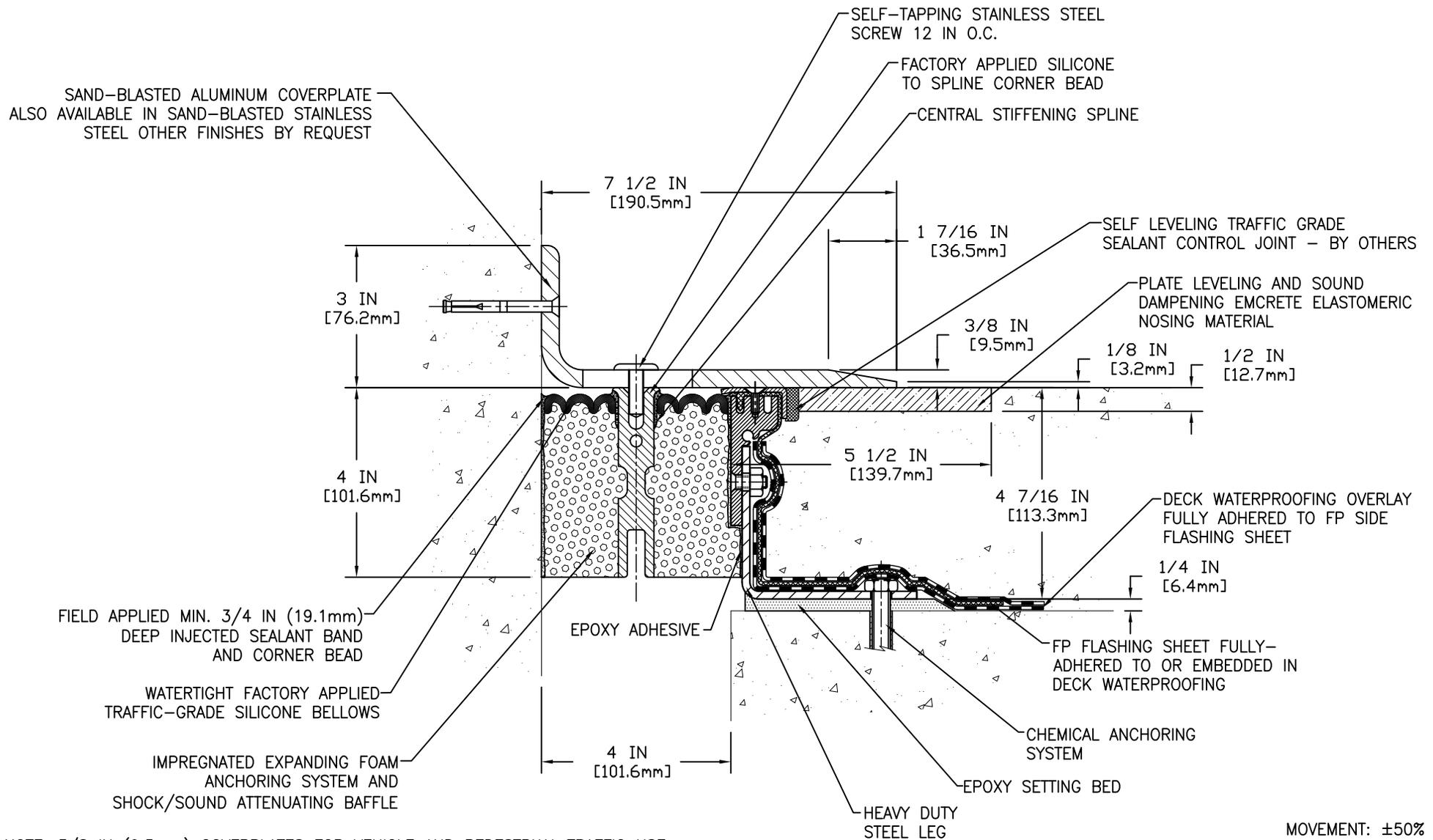
NOTE: 3/8 IN (9.5mm) COVERPLATES FOR VEHICLE AND PEDESTRIAN-TRAFFIC USE
