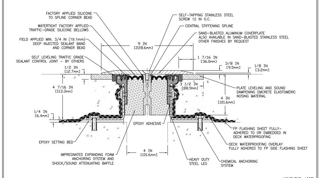
NOTE: 3/8 IN (9.5mm) COVERPLATES FOR VEHICLE AND PEDESTRIAN—TRAFFIC USE (FOR PEDESTRIAN—TRAFFIC ONLY, USE 1/4 IN (6.4mm) COVERPLATE)
