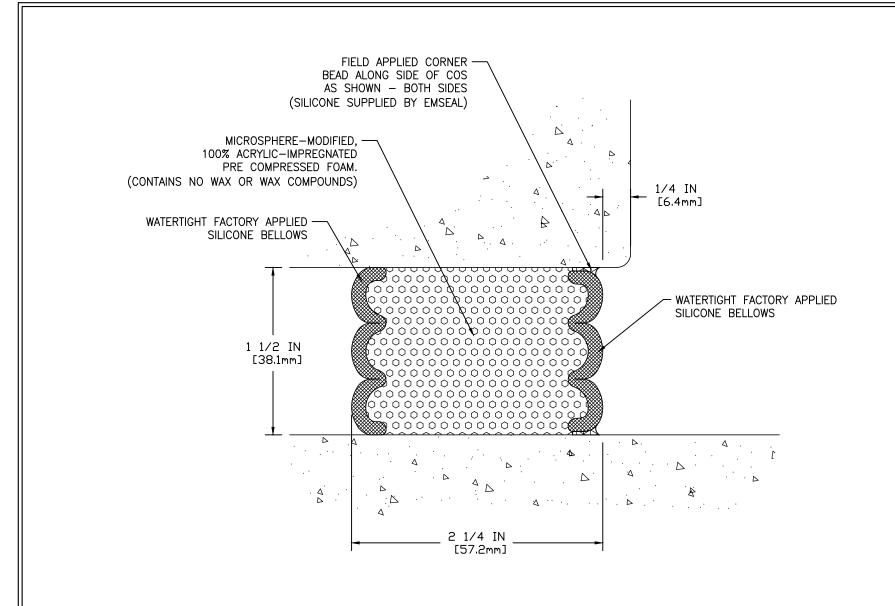
MOVEMENT: ±50% + 3/4 IN (20mm) - 3/4 IN (20mm)
