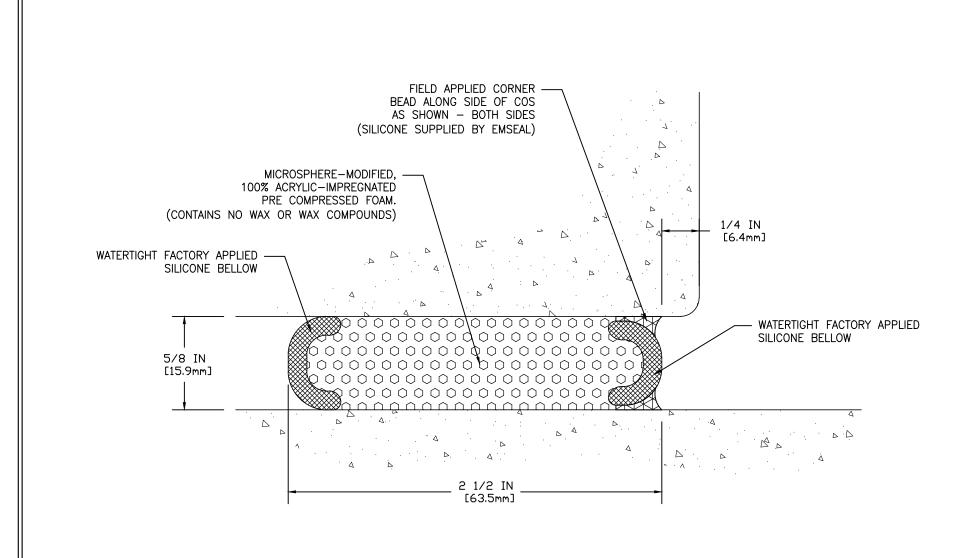
MOVEMENT: ±50% + 5/16 IN (8mm) - 5/16 IN (8mm)
