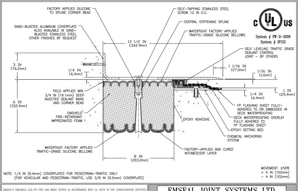
IN SYSTEM # FW-D-2009. USE OF THIS MATERIAL IN WALL ASSEMBLY CONFIGURATIONS OTHER THAT DEPICTED IN UL SYSTEM # FW-D-2009 WILL NOT ENCUMBER OR LOWER THE RESISTANCE OF THE WALL BUT IS DONE SO AT THE DESIGNERS' DISCRETION AND RESPONSIBILITY FOR DESIGN OF A FIRE RATED WALL ASSEMBLY THAT MEETS APPLICABLE STANDARDS FOR THE PROJECT AND WHICH ADDITIONALLY IS CAPABLE OF RESISTING THE APPROXIMATELY 2.5 PSI (120 LBS PER FOOT OF JOINT BASED ON 4-INCH DEPTH OF SEAL) BACKPRESURE OF THE SJS-FP-FR2 MATERIAL.
