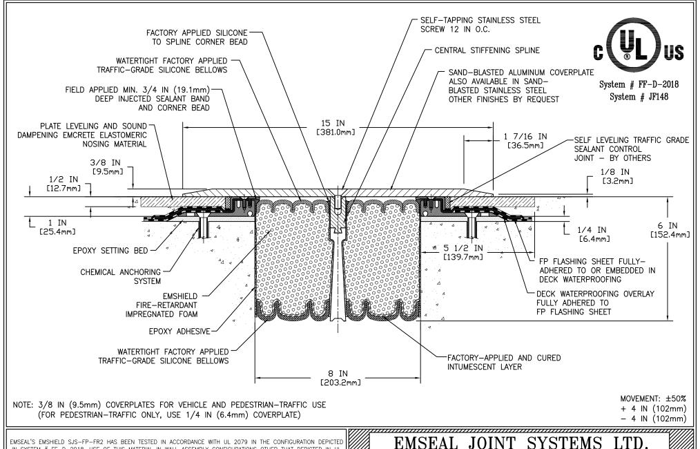
IN SYSTEM # FF-D-2018. USE OF THIS MATERIAL IN WALL ASSEMBLY CONFIGURATIONS OTHER THAT DEPICTED IN UL SYSTEM #"FF-D-2018 WILL NOT ENCUMBER OR LOWER THE RESISTANCE OF THE WALL BUT IS DONE SO AT THE DESIGNERS' DISCRETION AND RESPONSIBILITY FOR DESIGN OF A FIRE RATED WALL ASSEMBLY THAT MEETS APPLICABLE STANDARDS FOR THE PROJECT AND WHICH ADDITIONALLY IS CAPABLE OF RESISTING THE APPROXIMATELY 2.5 PSI (120 LBS PER FOOT OF JOINT BASED ON 4-INCH DEPTH OF SEAL) BACKPRESURE OF THE SJS-FP-FR2 MATERIAL.
