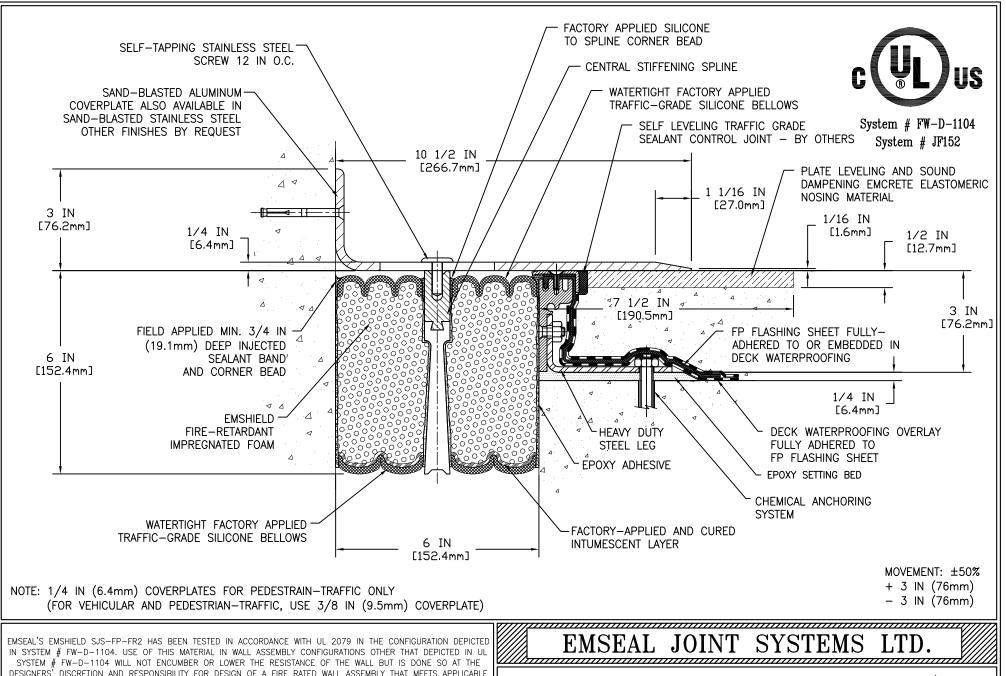
DESIGNERS' DISCRETION AND RESPONSIBILITY FOR DESIGN OF A FIRE RATED WALL ASSEMBLY THAT MEETS APPLICABLE STANDARDS FOR THE PROJECT AND WHICH ADDITIONALLY IS CAPABLE OF RESISTING THE APPROXIMATELY 2.5 PSI (120 LBS PER FOOT OF JOINT BASED ON 4-INCH DEPTH OF SEAL) BACKPRESURE OF THE SJS-FP-FR2 MATERIAL.
