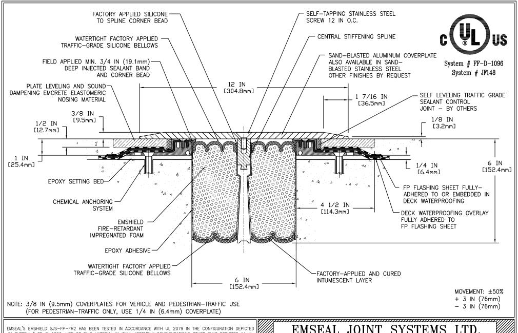
IN SYSTEM # FF-D-1096. USE OF THIS MATERIAL IN WALL ASSEMBLY CONFIGURATIONS OTHER THAT DEPICTED IN UL SYSTEM #"FF-D-1096 WILL NOT ENCUMBER OR LOWER THE RESISTANCE OF THE WALL BUT IS DONE SO AT THE DESIGNERS' DISCRETION AND RESPONSIBILITY FOR DESIGN OF A FIRE RATED WALL ASSEMBLY THAT MEETS APPLICABLE STANDARDS FOR THE PROJECT AND WHICH ADDITIONALLY IS CAPABLE OF RESISTING THE APPROXIMATELY 2.5 PSI (120 LBS PER FOOT OF JOINT BASED ON 4-INCH DEPTH OF SEAL) BACKPRESURE OF THE SJS-FP-FR2 MATERIAL.
