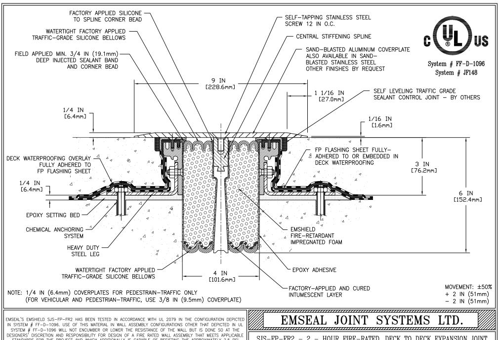
STANDARDS FOR THE PROJECT AND WHICH ADDITIONALLY IS CAPABLE OF RESISTING THE APPROXIMATELY 2.5 PSI (120 LBS PER FOOT OF JOINT BASED ON 4-INCH DEPTH OF SEAL) BACKPRESURE OF THE SJS-FP-FR2 MATERIAL.
