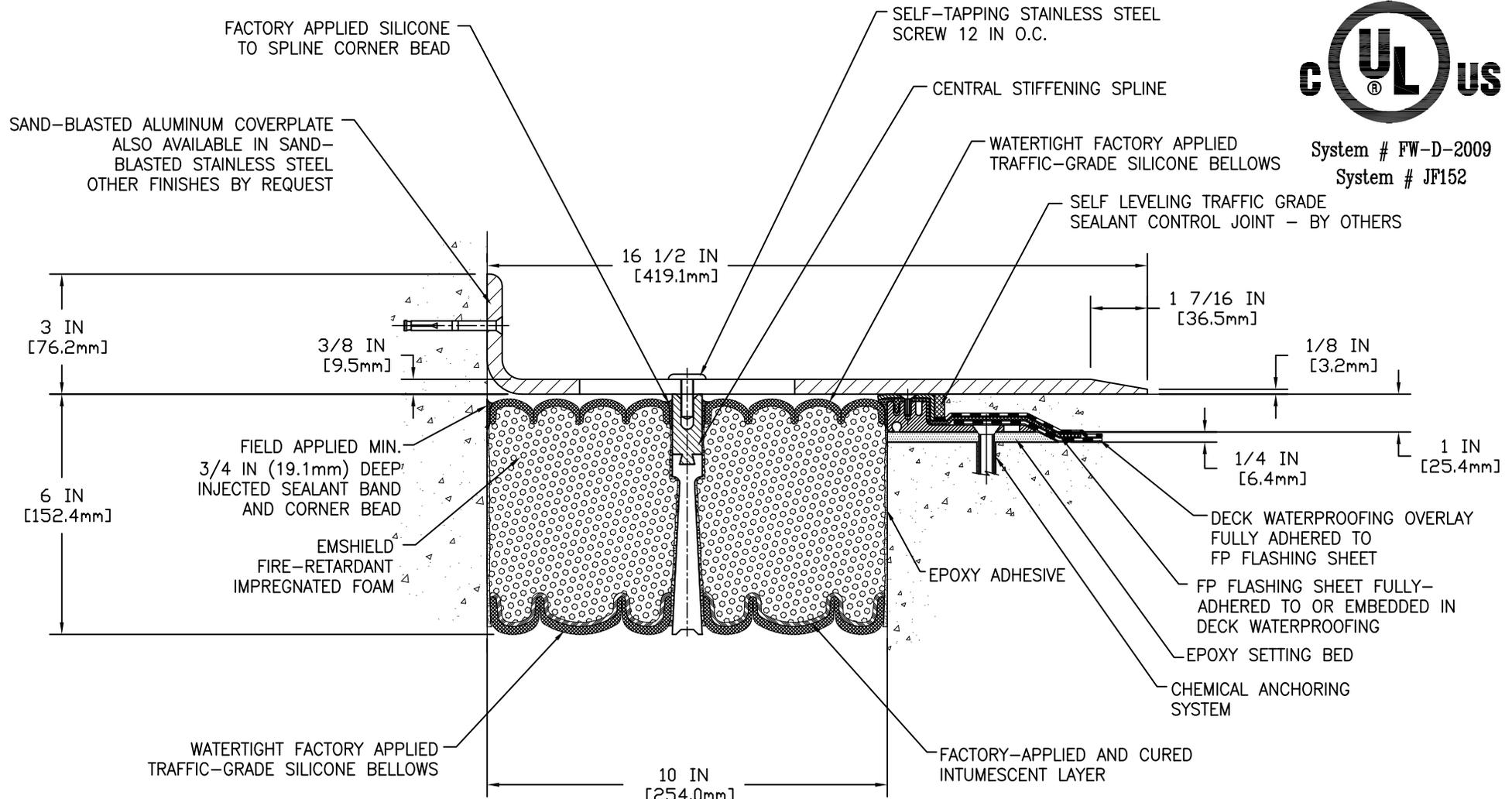
NOTE: 3/8 IN (9.5mm) COVERPLATES FOR VEHICLE AND PEDESTRIAN-TRAFFIC USE
