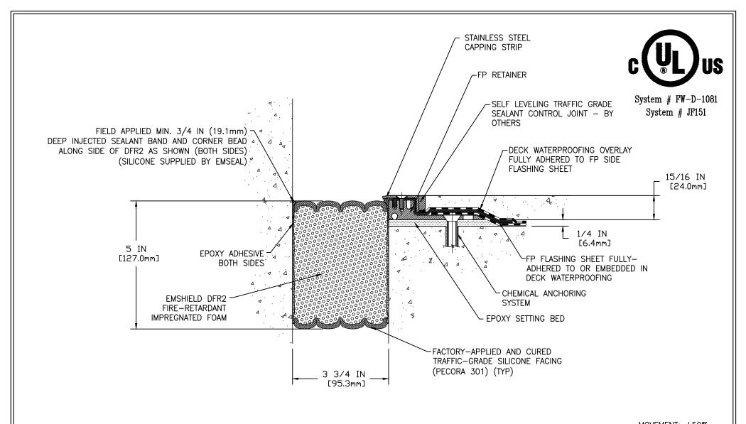
MOVEMENT: ±50% + 1 7/8 IN (48mm) - 1 7/8 IN (48mm)
