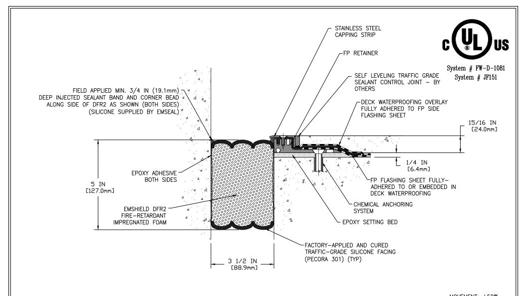
MOVEMENT: ±50% + 1 3/4 IN (45mm) - 1 3/4 IN (45mm)
