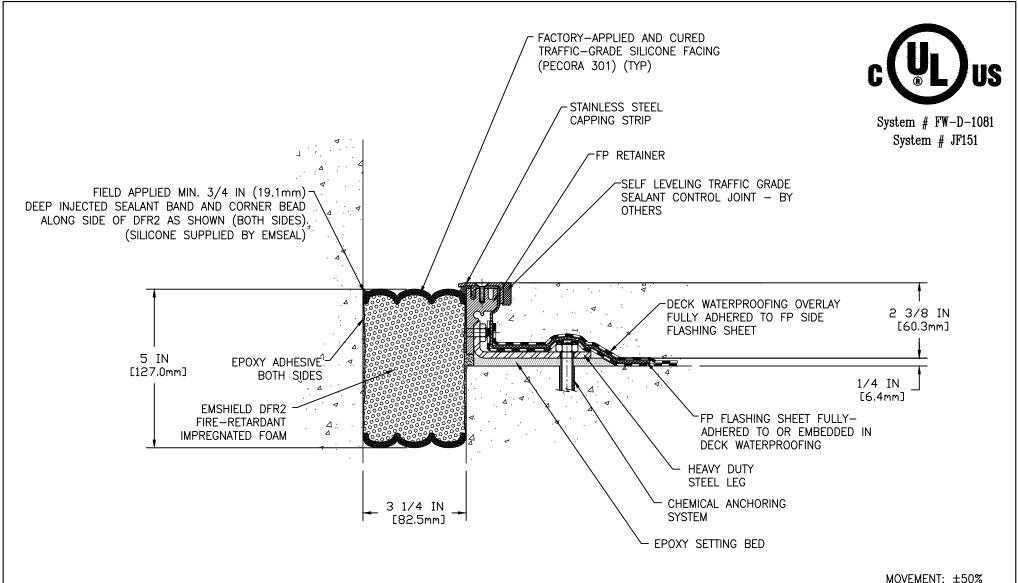
MOVEMENT: ±50% + 1 5/8 IN (42mm) - 1 5/8 IN (42mm)
