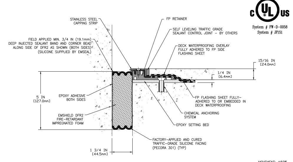
MOVEMENT: ±50% + 7/8 IN (22mm) - 7/8 IN (22mm)
