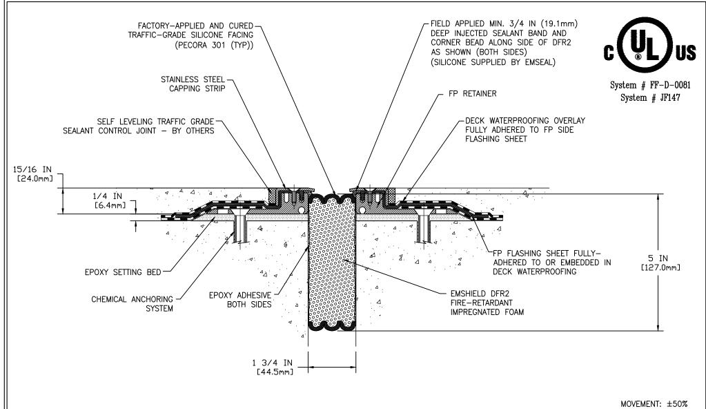
MOVEMENT: ±50% + 7/8 IN (22mm) - 7/8 IN (22mm)
