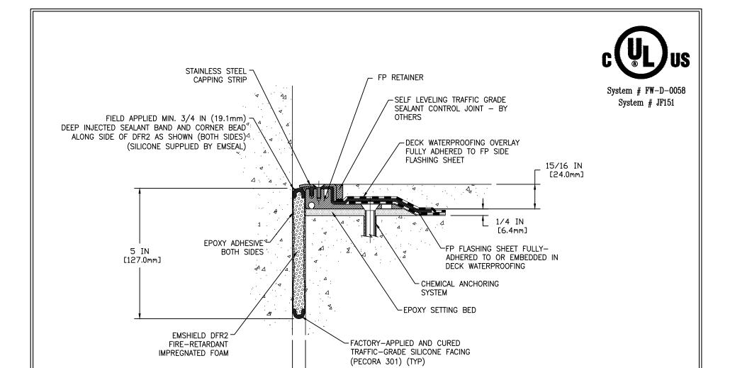
MOVEMENT: ±50% + 1/4 IN (6mm) - 1/4 IN (6mm)
