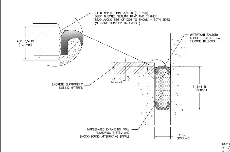
MOVEMENT: ±50% + 1/2 IN (13mm) - 1/2 IN (13mm)
