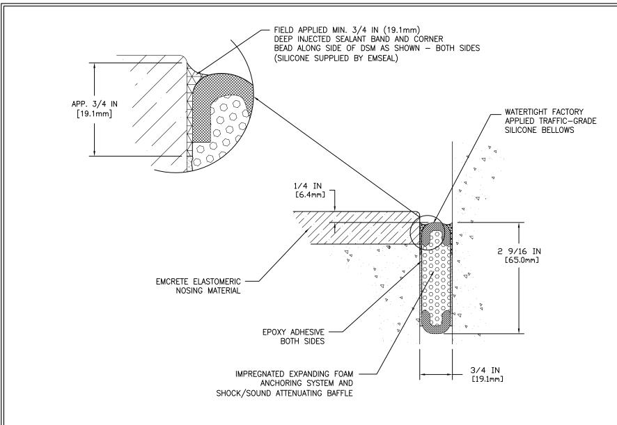
MOVEMENT: ±50% + 3/8 IN (10mm) - 3/8 IN (10mm)
