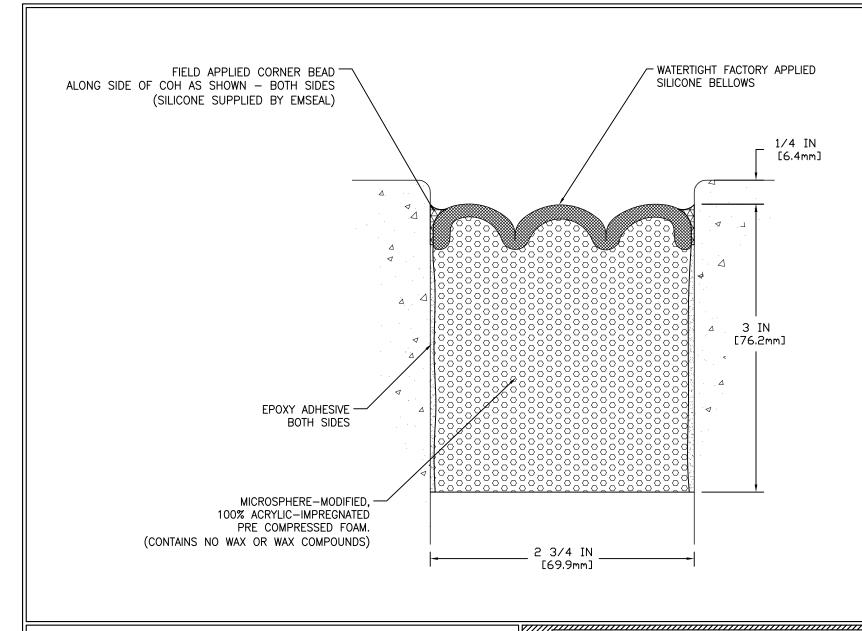
MOVEMENT: ±50% + 1 3/8 IN (35mm) - 1 3/8 IN (35mm)
