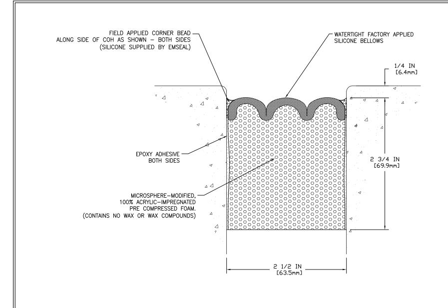
MOVEMENT: ±50% + 1 1/4 IN (32mm) - 1 1/4 IN (32mm)
