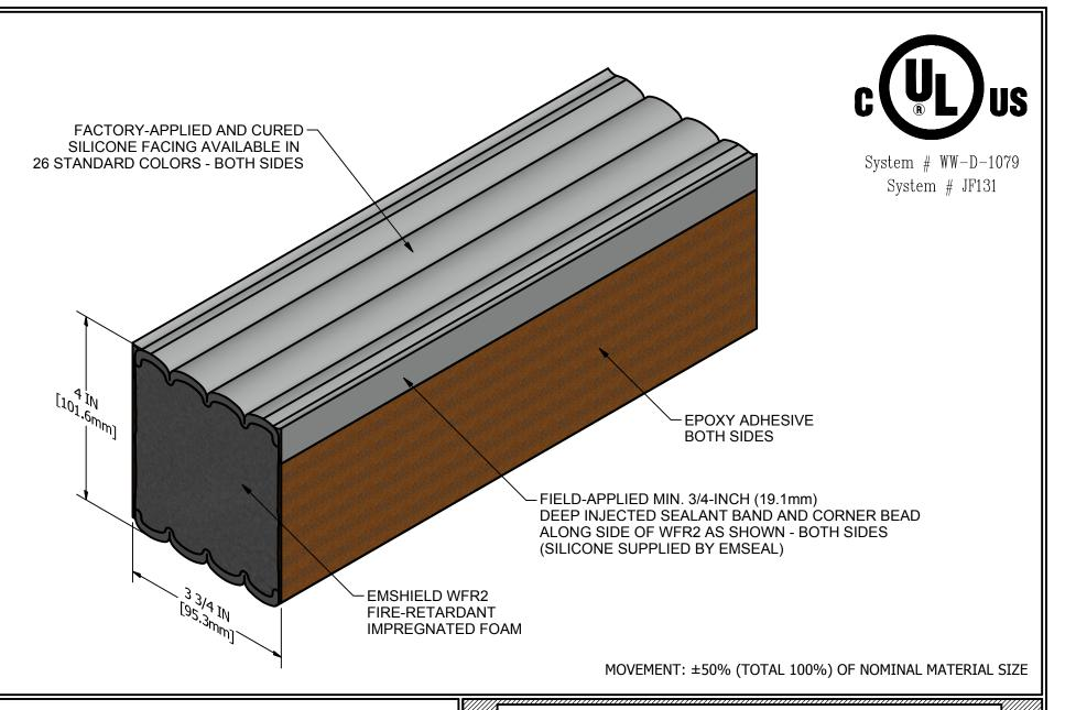
EMSEAL'S EMSHIELD WFR2 HAS BEEN TESTED IN ACCORDANCE WITH UL 2079 IN THE CONFIGURATION THAT DEPICTED IN UL SYSTEM # WW-D-1079 WILL NOT ENCUMBER OR LOWER THE RESISTANCE OF THE WALL BUT IS DONE SO AT THE DESIGNERS' DISCRETION AND RESPONSIBILITY FOR DESIGN OF A FIRE RATED WALL ASSEMBLY THAT MEETS APPLICABLE STANDARDS FOR THE PROJECT AND WHICH ADDITIONALLY IS CAPABLE OF RESISTING THE APPROXIMATELY 2.5 PSI (120 LBS PER FOOT OF JOINT BASED ON 4-INCH DEPTH OF SEAL) BACKPRESURE OF THE WFR2 MATERIAL.
