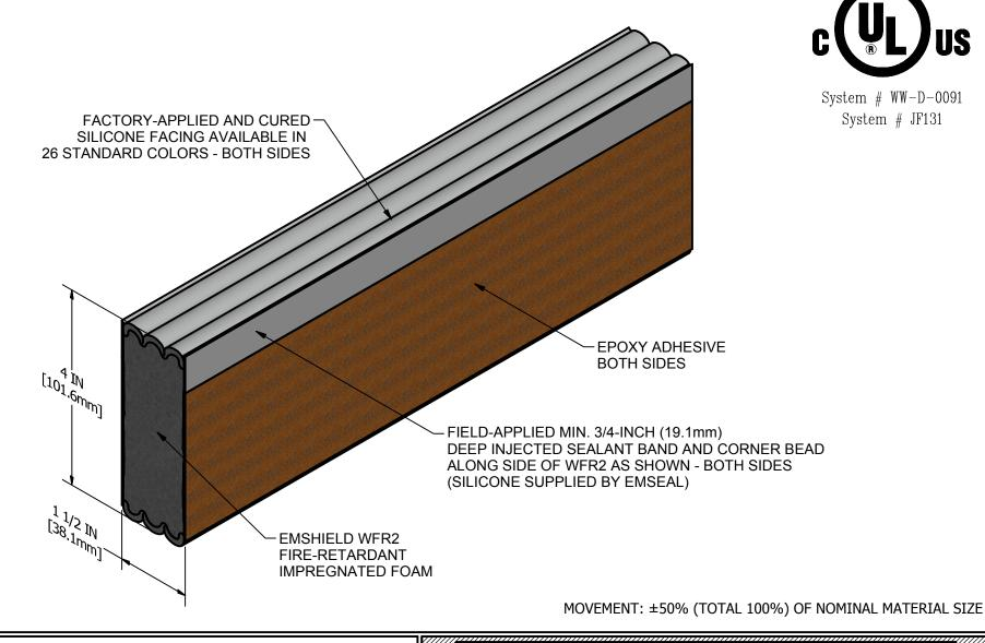
EMSEAL'S EMSHIELD WFR2 HAS BEEN TESTED IN ACCORDANCE WITH UL 2079 IN THE CONFIGURATION THAT DEPICTED IN UL SYSTEM # WW-D-0091 WILL NOT ENCUMBER OR LOWER THE RESISTANCE OF THE WALL BUT IS DONE SO AT THE DESIGNERS' DISCRETION AND RESPONSIBILITY FOR DESIGN OF A FIRE RATED WALL ASSEMBLY THAT MEETS APPLICABLE STANDARDS FOR THE PROJECT AND WHICH ADDITIONALLY IS CAPABLE OF RESISTING THE APPROXIMATELY 2.5 PSI (120 LBS PER FOOT OF JOINT BASED ON 4-INCH DEPTH OF SEAL) BACKPRESURE OF THE WFR2 MATERIAL.
