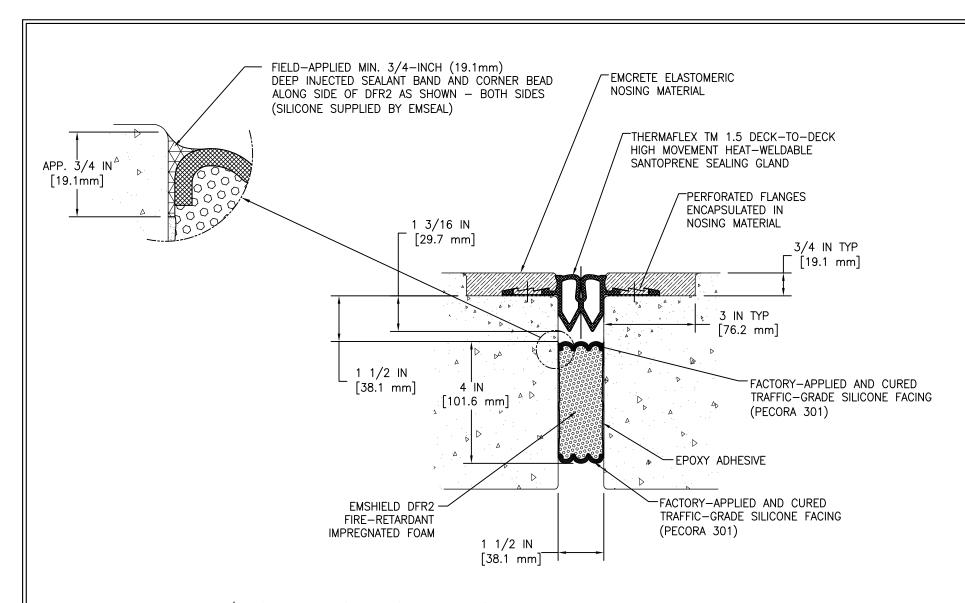
THERMAFLEX TM 1.5 MOVEMENT: 1/2 INCH MIN JOINT GAP-3 INCH MAX JOINT GAP EMSHIELD DFR2 MOVEMENT: ±50% (TOTAL 100%) OF NOMINAL MATERIAL SIZE
