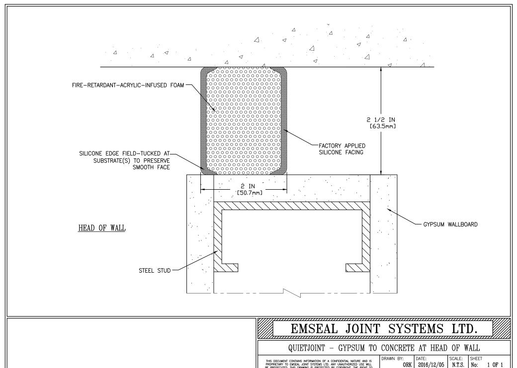
THIS DOCUMENT CONTAINS INFORMATION OF A CONFIDENTIAL NATURE AND IS PROPRIETARY TO EMISEAL JOINT SYSTEMS LTD. ANY UNAUTHORIZED USE WILL BE PROSECUTED. THIS DRAWING IS PROTICCTED BY COPYRIGHT, THE RIGHT TO REPRODUCE IN ANY FORM BEING THE EXCLUSIVE RIGHT OF EMISEAL JOINT SYSTEMS LTD. ANY UNAUTHORIZED REPRODUCTION WHETHER IN TWO OR THREE DIMENSIONS WILL BE PROSECUTED. © 2014 EMISEAL JOINT SYSTEMS LTD.
