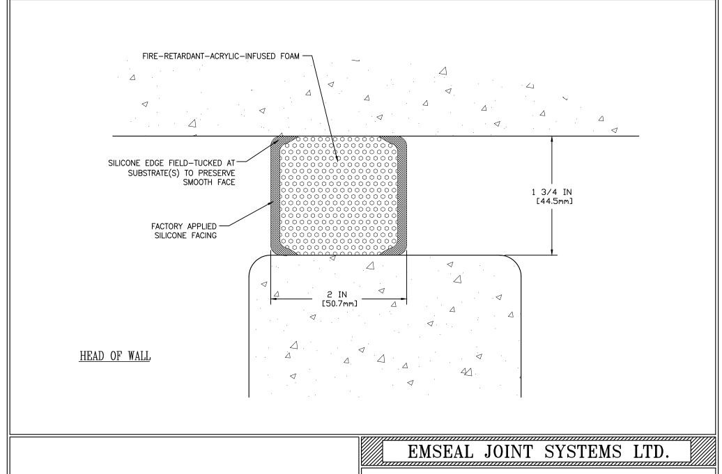
QUIETJOINT - CONCRETE TO CONCRETE AT HEAD OF WALL
