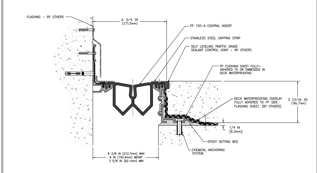
MOVEMENT: ±50% + 2 3/8 IN (60mm) - 2 3/8 IN (60mm)
