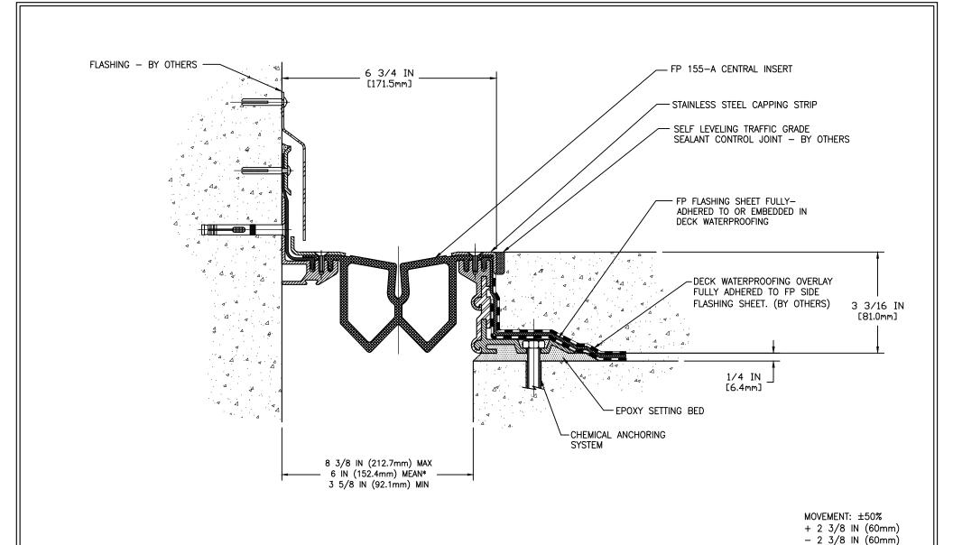
\* - MEAN JOINT WIDTH 6 IN (152.4mm)
