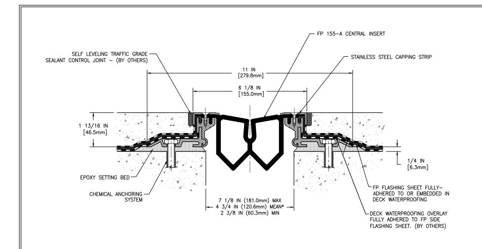
MOVEMENT: ±50% + 2 3/8 IN (60mm) - 2 3/8 IN (60mm)
