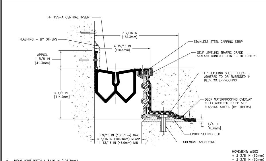
\* - MEAN JOINT WIDTH 4 3/16 IN (106.4mm)
