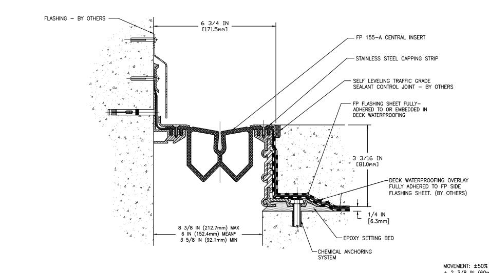
\* - MEAN JOINT WIDTH 6 IN (152.4mm)
