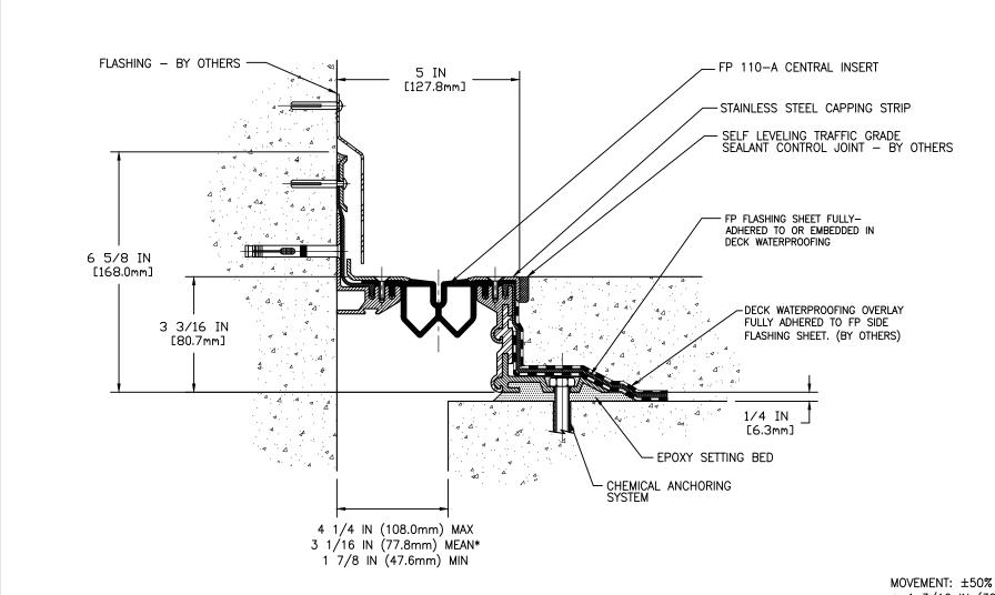
\* - MEAN JOINT WIDTH 3 1/16 IN (77.8mm)
