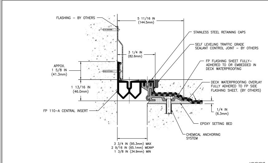
\* - MEAN JOINT WIDTH 2 9/16 IN (65.1mm)
