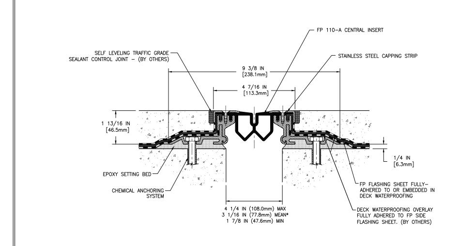
\* - MEAN JOINT WIDTH 3 1/16 IN (77.8mm)
