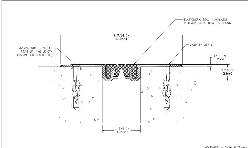
MOVEMENT: + 3/16 IN (5mm) - 3/16 IN (5mm)
