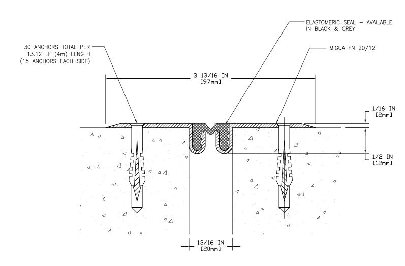
MOVEMENT: + 1/8 IN (3mm) - 1/16 IN (2mm)
