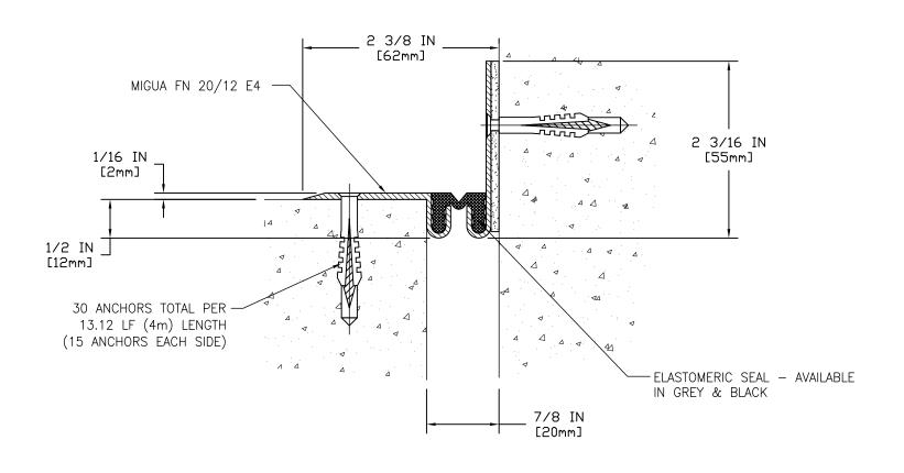
MOVEMENT: + 1/8 IN (3mm) - 1/8 IN (3mm)
