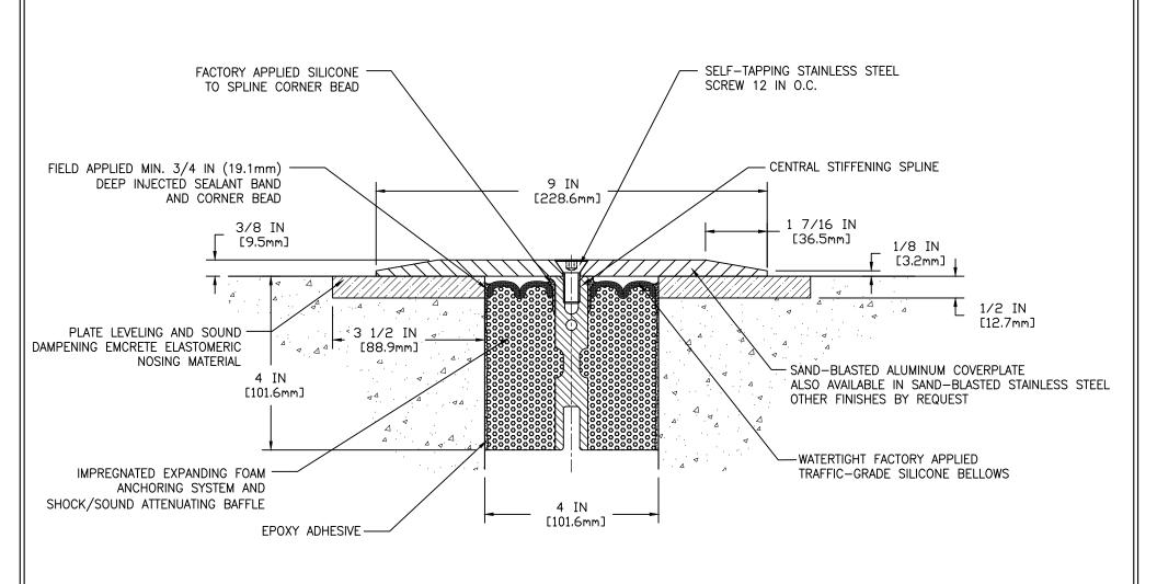
NOTE: 3/8 IN (9.5mm) COVERPLATES FOR VEHICLE AND PEDESTRIAN-TRAFFIC USE (FOR PEDESTRIAN-TRAFFIC ONLY, USE 1/4 IN (6.4mm) COVERPLATE)
