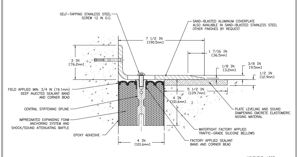
NOTE: 3/8 IN (9.5mm) COVERPLATES FOR VEHICLE AND PEDESTRIAN—TRAFFIC USE (FOR PEDESTRIAN—TRAFFIC ONLY, USE 1/4 IN (6.4mm) COVERPLATE)
