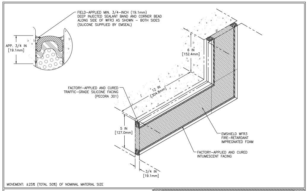
EMSEAL'S EMSHIELD WFR3 HAS BEEN TESTED IN ACCORDANCE WITH UL 2079 IN THE CONFIGURATION DEPICTED IN SYSTEM # WW-D-0099. USE OF THIS MATERIAL IN WALL ASSEMBLY CONFIGURATIONS OTHER THAT DEPICTED IN UL SYSTEM # WW-D-0099 WILL NOT ENCUMBER OR LOWER THE RESISTANCE OF THE WALL BUT IS DONE SO AT THE
